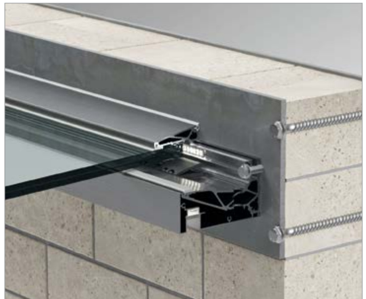
ANCHORING TO BEARING STRUCTURE IN MASONRY WITH PARTITION PLATE canopy with functional lighting cover
