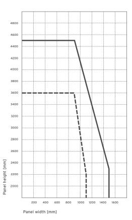
Applies to fill-ins/glazing max. 20 kg/m² / double glazing
